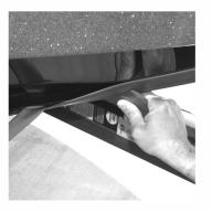
Once fully attached, use the burnishing tool to apply additional pressure to the entire KeelGuard ensuring the pressure sensitive adhesive is firmly attached to the boat. A rubber mallet may also be used to apply even more force to the 3M
